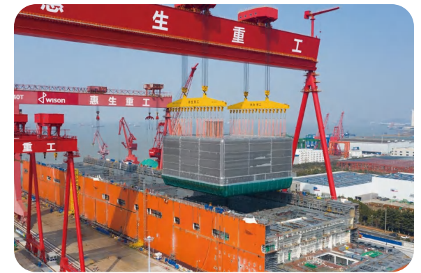
The World's Largest SPB® Tank Built at WNE Nantong Yard
